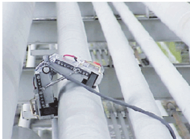
Fig.8: EMAT on a pipeline.
