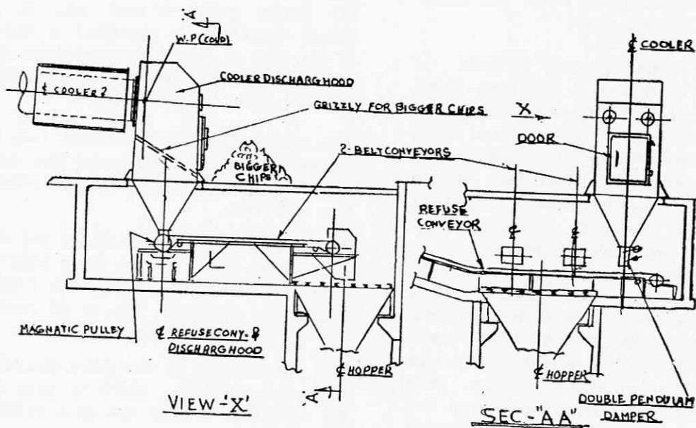
Fig 4 Cooler Discharge Arrangement
