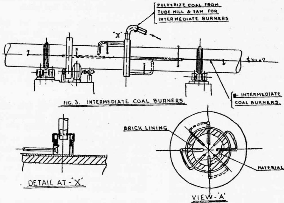
Fig. 3 Intermediate Coal Burners.
