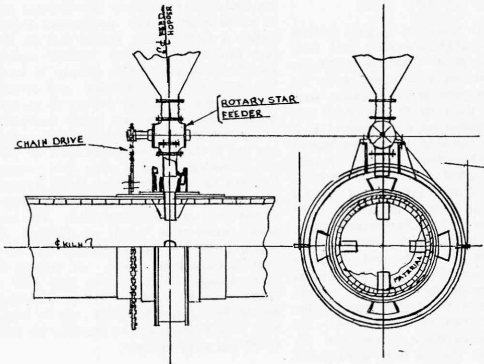
Fig. 2 Coal Throwing arrangement
