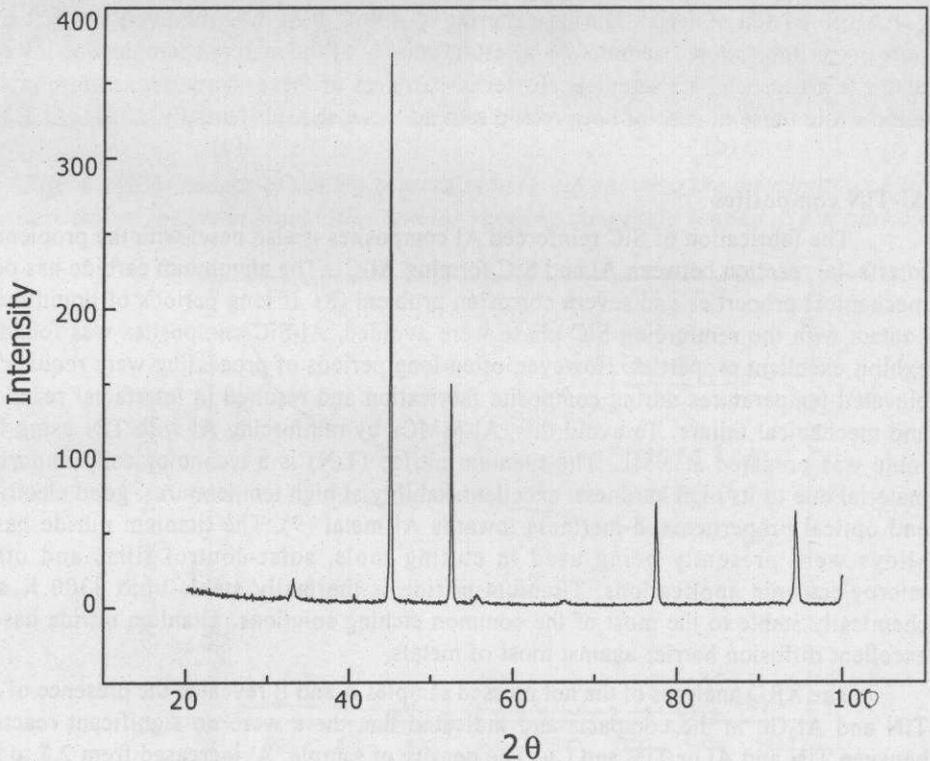
Fig. 3 : XRD pattern of Al-SiC Composite powder
