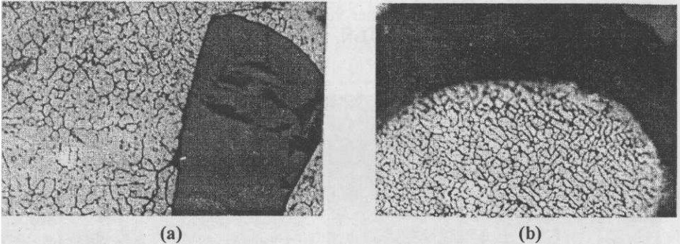
Fig.6 : Optical micrographs of over sprayed powder (a) Al-rutile and (b) Al-2Mg alloy X500
