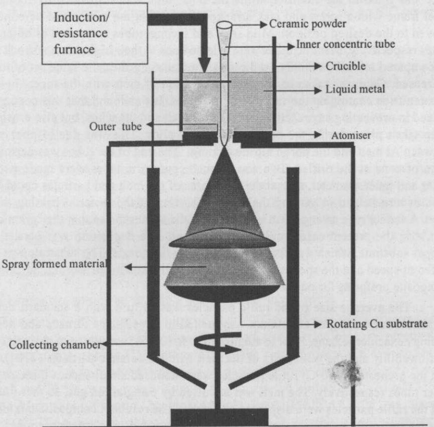
Fig. 2: Schematic diagram of spray forming set-up for preparation of Al-TiO<sub>2</sub> composites
