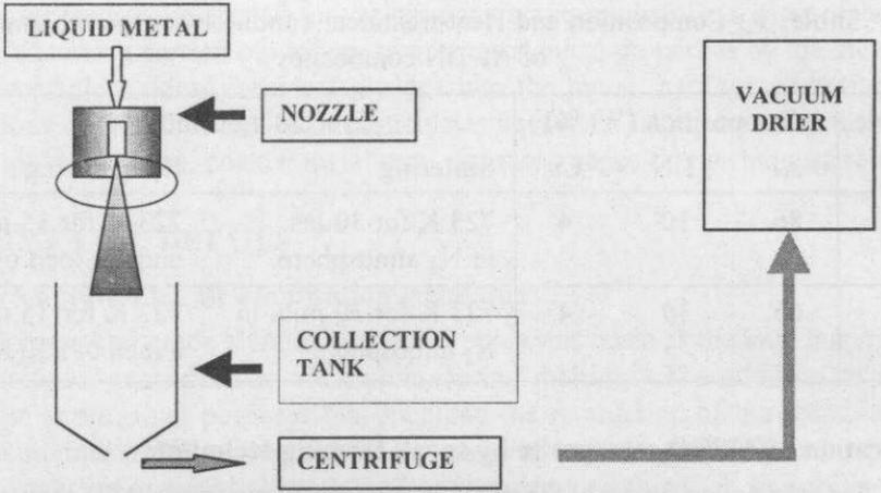
Fig. 1 : Schematic diagram of air atomisation process
