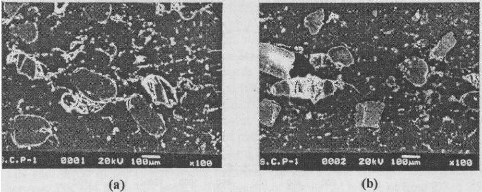
Fig.7 : SEM photomicrograph of as spray formed Al-2Mg-11TiO<sub>2</sub> composite at locations a) centre and b) at periphery
