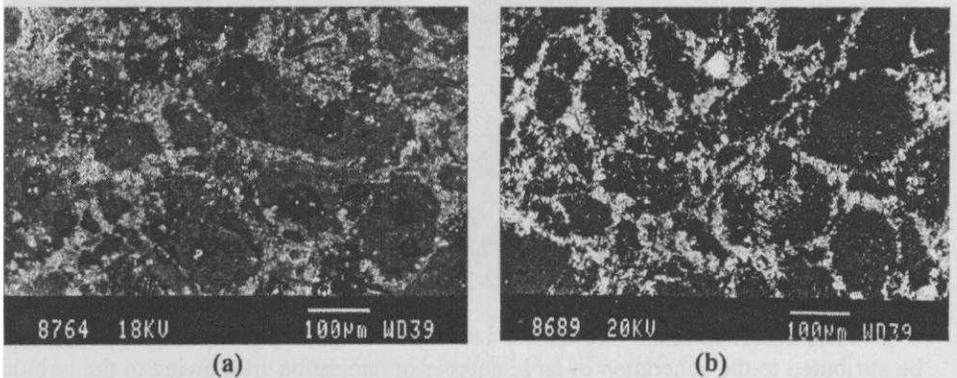
Fig. 4 : SEM images of the hot pressed sample; (a) showing the distribution of TiN particles at the grain boundaries and (b) showing the needle shaped  $Al_2Cu$  particles
