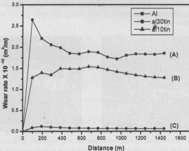
Fig.5 : Wear rate of (a) Al, (b) Al-10TiN and (c) Al-30TiN
