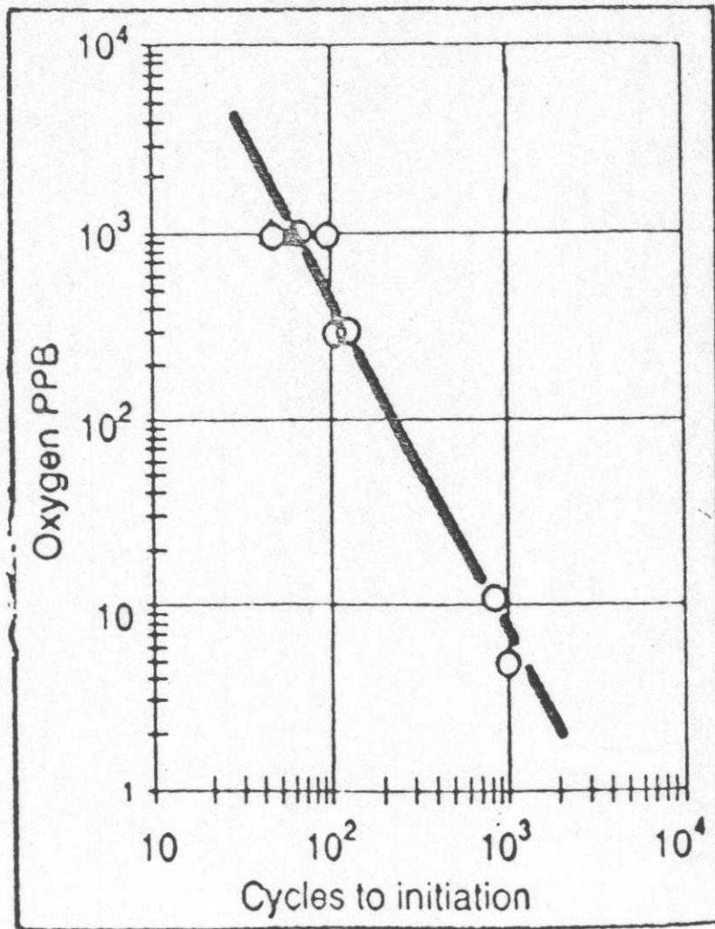
Figure 7 Corrosion fatigue Initiation as a function of boiler water dissolved oxygen content.
