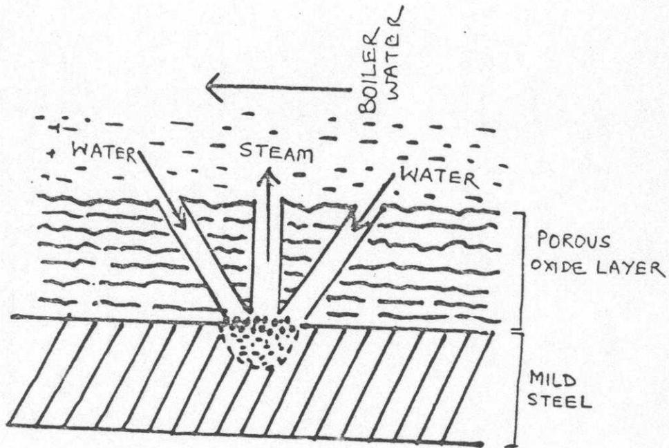
Figure-I Mechanism of Salt Concentration by Wick Boiling Phenomenon Inside the Internal Deposit
