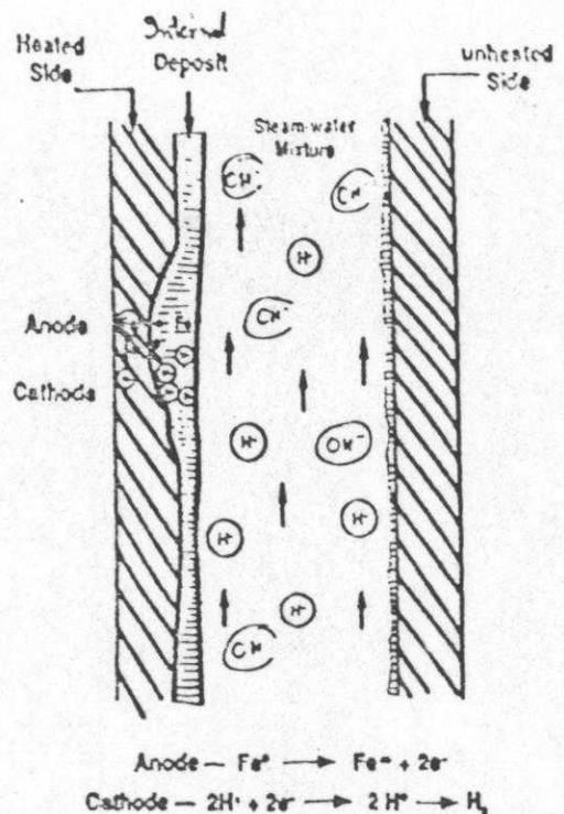
Figure-V: Mechanism of Formation of Acidic Condition Inside the Internal Deposit in Water Wall Tube
