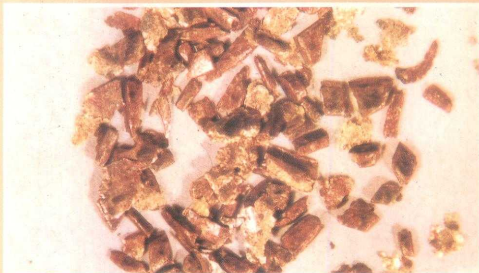
Megascopic view of Par-Heavy fraction from Purulia region shows the presence of gold in the sample
