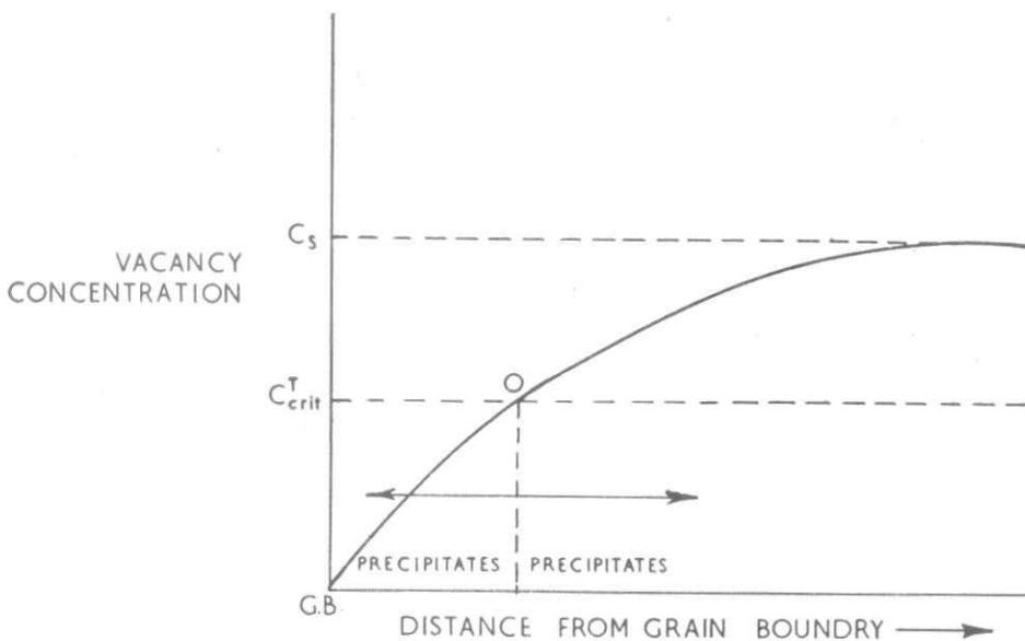
1 A schematic illustration of the vacancy concentration profile formed on quenching.  $C^S$  is the equilibrium vacancy concentration at the solution temperature  $T_S$  and  $C^{T_{crit}}$  is the critical vacancy concentration required to nucleate precipitates at an aging temperature  $T$  (From J. D. Embury and R. B. Nicholson).
