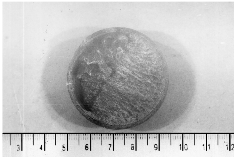
Fig. 4. Macrograph of the fracture surface of the failed stud.
