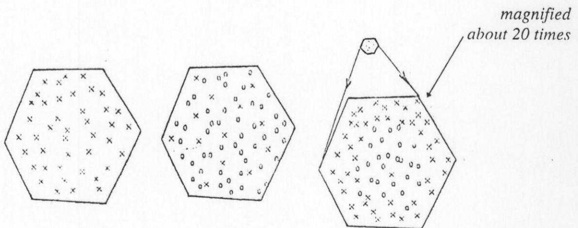
Fig. 3: Schematic GP-zone structure in the alloys investigated
