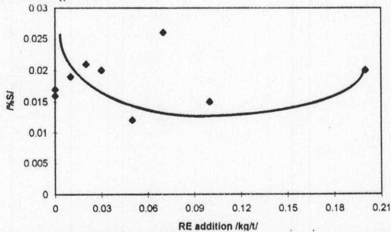
Figure 1. Relationship between RE addition amount and residual sulphur content in steel
