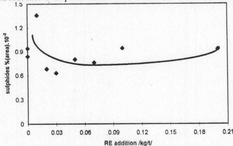
Figure 2. Affect of RE addition on sulphide quantity in the steel.
