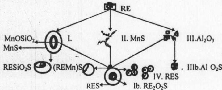
**Figure 6.** Schematic of modification of the inclusions in steel containing RE
