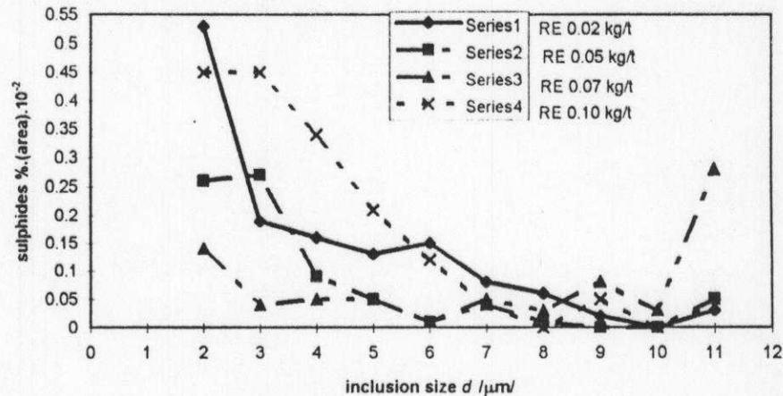
Figure 3. Relationship between sulphide sizes and sulphide amounts in steel products on RE amount additions
