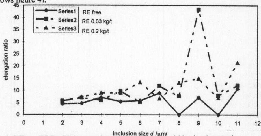
Figure 4. Effect of RE addition on elongation ratio of sulphides in pipe steel
