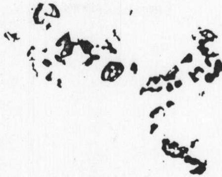
**Figure 5.** Optical micrograph of inclusions in steel before addition of RE, x500
