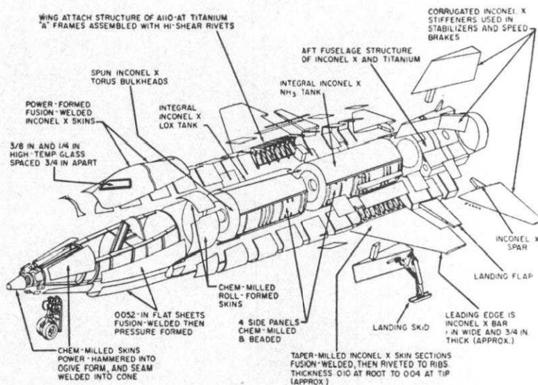
Exploded view showing material of construction
