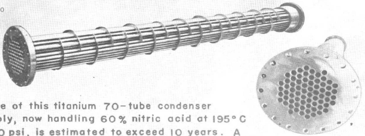
The life of this titanium 70-tube condenser assembly, now handling 60% nitric acid at 195° C and 180 psi, is estimated to exceed 10 years. A similar stainless assembly would last 4 months
