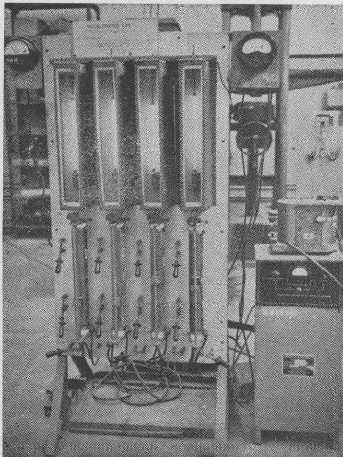
6 Accelerated life testing apparatus
