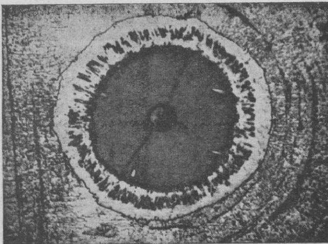
23 Ni-B composite after exposure at 1380° F for 1 hour X500
