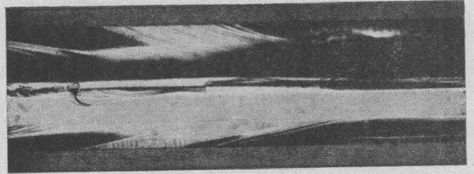
10 View of longitudinal forced crack in a boron filament with conchoidal fracture lines  $\times 300$
