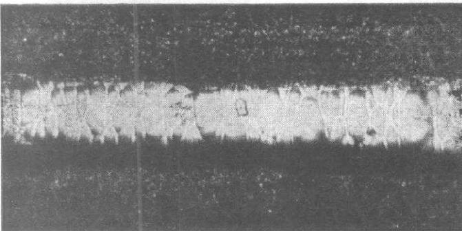
(c) Surface of nickel matrix showing replication of boron surface  $\times 340$
