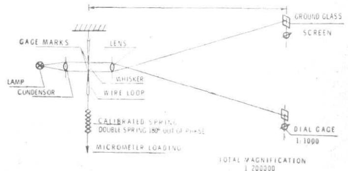
15 Schematic diagram of the tensile tester
