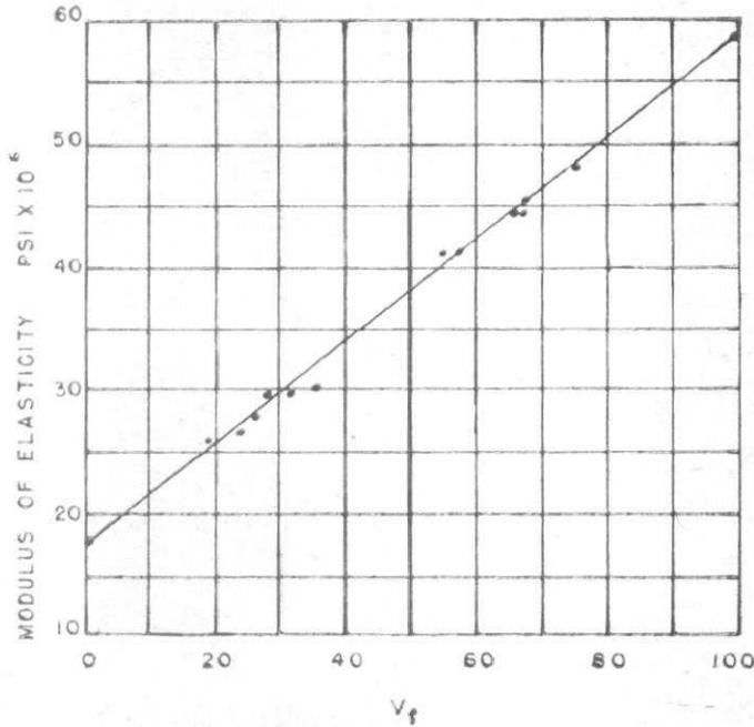
1 Dynamic modulus of elasticity of tungsten, copper, and copper reinforced with tungsten wires (McDANIELS ET AL (4))
