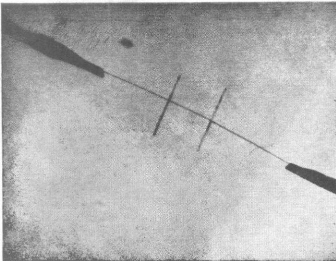
13 Gage marks on whisker cemented to a wire loop ×15
