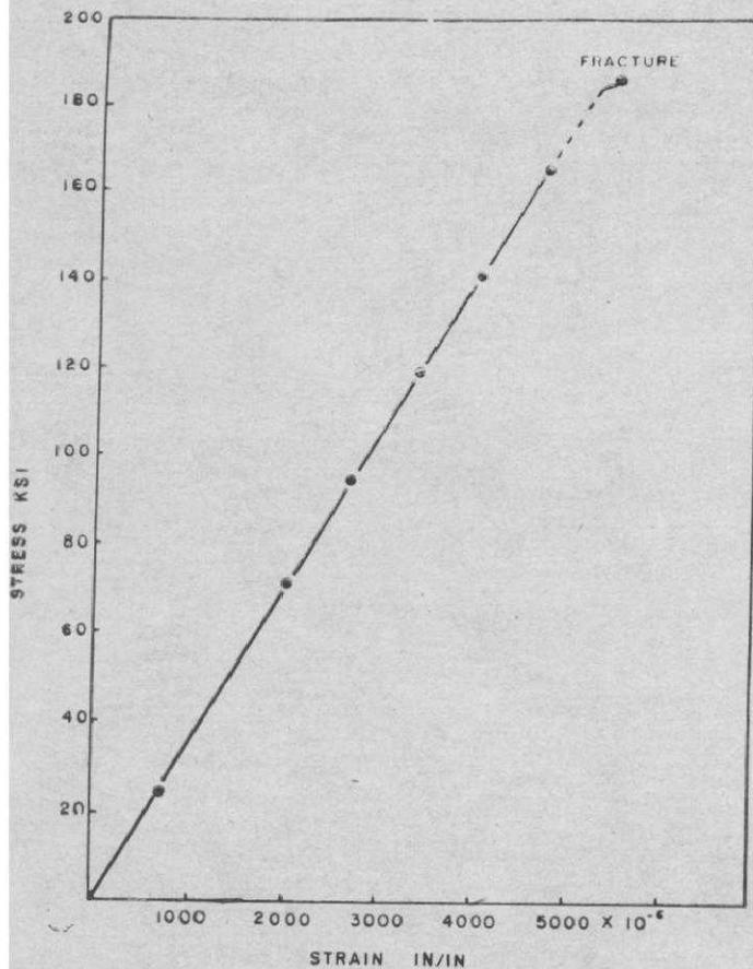
17 Stress-strain curve of iron whisker as obtained on the whisker tensile tester (Cross section at fracture =  $3.3 \mu^2$  used to calculate stress)
