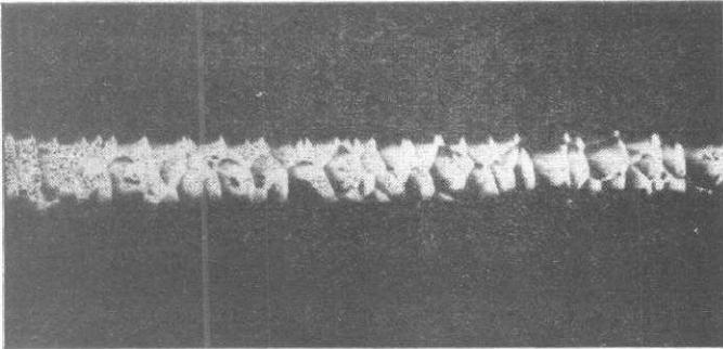
(b) Surface of boron filament  $\times 340$
