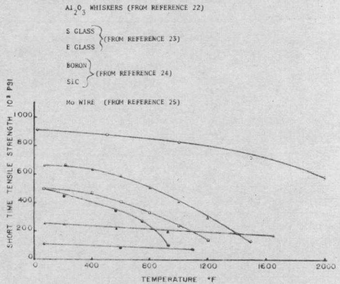
4 Filament strength as a function of temperature
