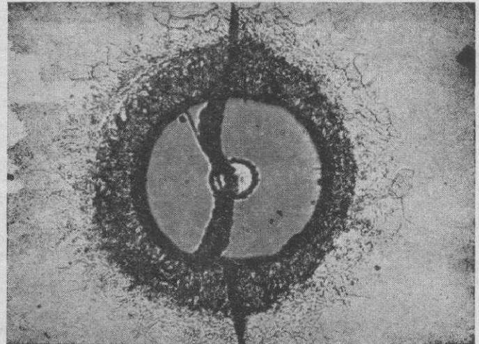
25 Maraging steel (Fe-18Ni)—boron composite after exposure at 1650°F for 1 hour X500
