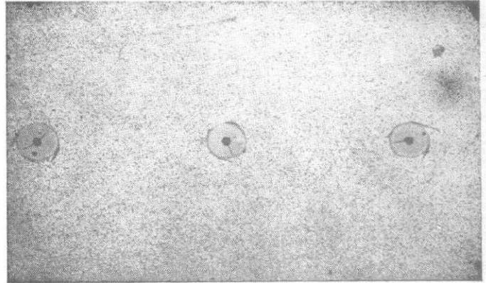
20 Illustration of metallurgical bond in a Ti-6Al-4V-Boron composite (Courtesy NAA/LAD)  $\times 100$
