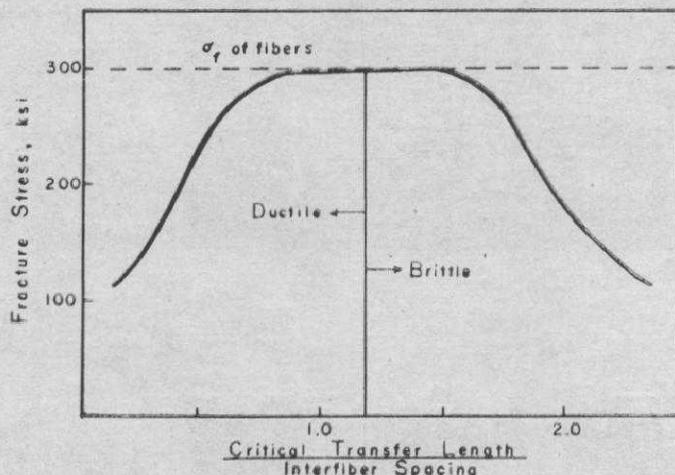
5 Effect of critical transfer length and interfiber spacing on fracture and type of fracture in steel wire-lead solder composites (Parikh 17)
