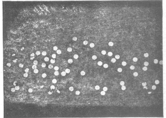
3 Macrostructure of aluminium-boron composite which exhibits fiber reinforcement  $\times 25$
