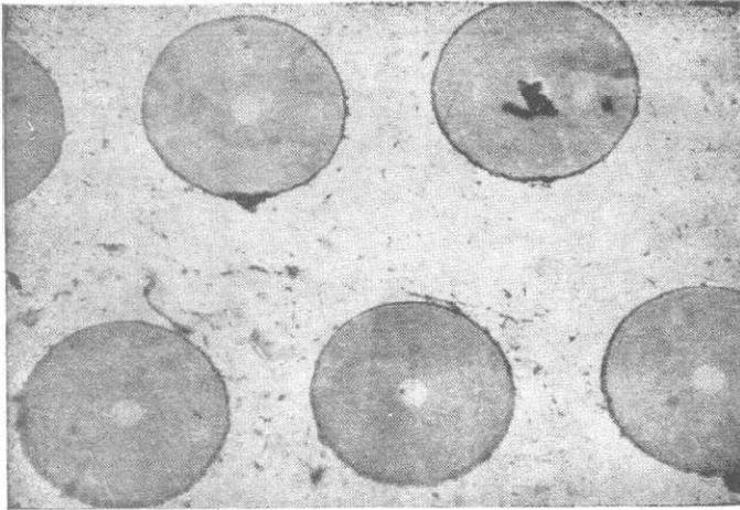
(a) Boron fibers embedded in a nickel matrix  $\times 250$
