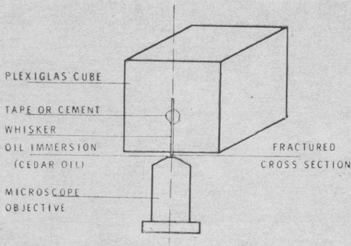
16 Arrangement of the fractured whisker for measurement of the area under the microscope (Schematic)
