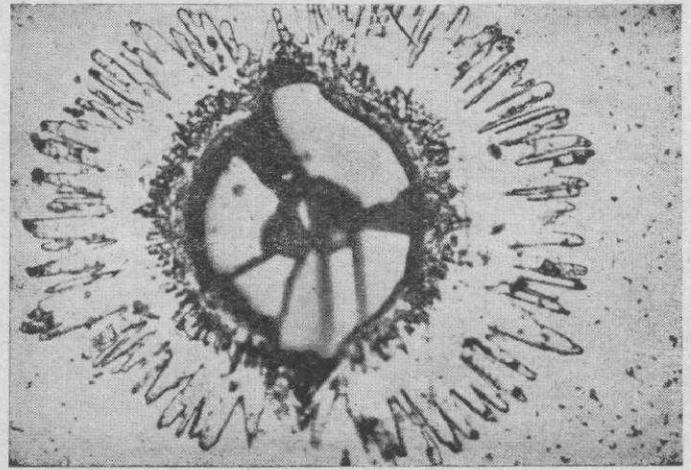
24 Fe-B Composite after exposure at 1650°F for 1 hour
