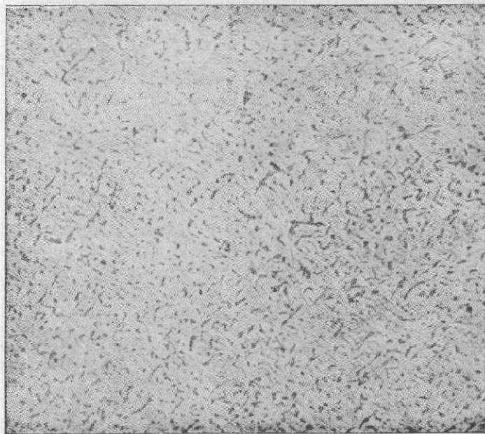
16 After tempering at 600°C for 200 hr.
