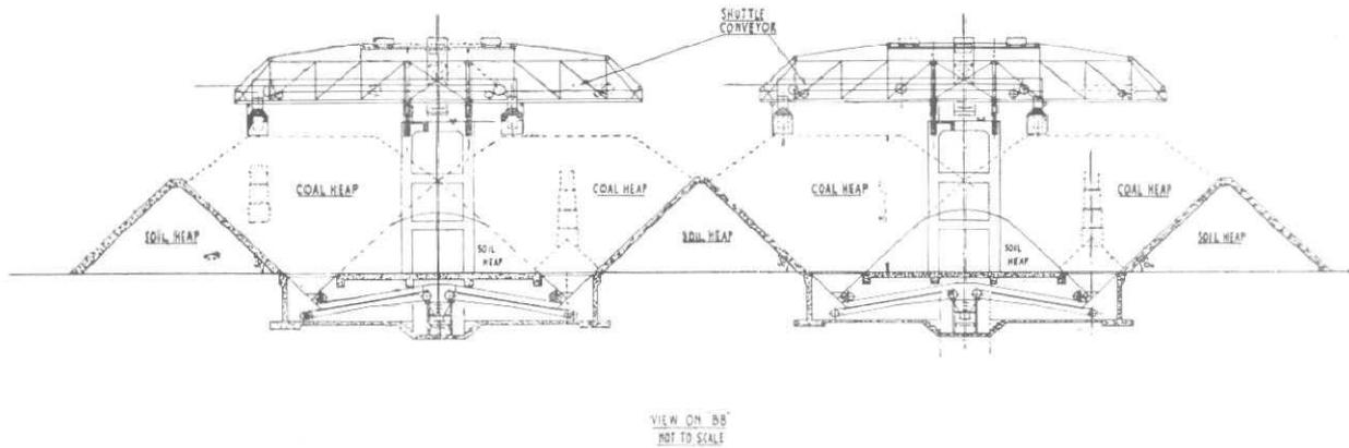
Arrangement of stacking and reclaiming in the ground storage.
