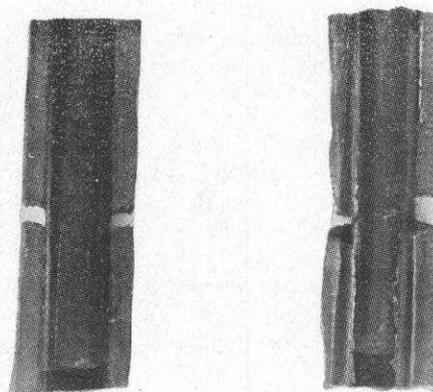
(b) Longitudinal section showing loose adhesion.
