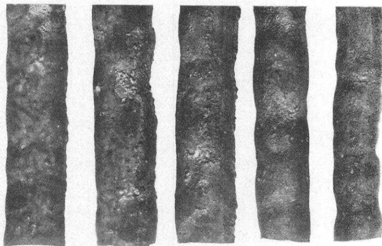
(a) Surface undulation of adhered metal.
