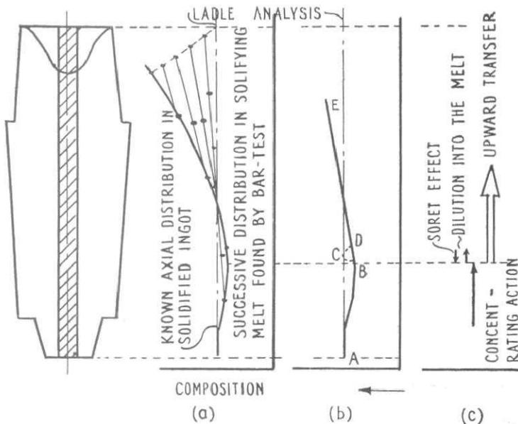
FIG. 18 MECHANISM OF VERTICAL SEGREGATION.
