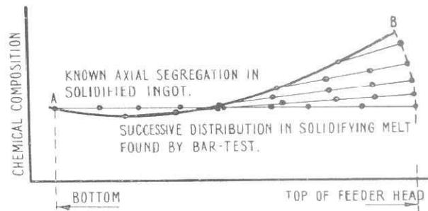
FIG. 8 AXIAL SEGREGATION AS RELATED TO THE RESULT OF ANALYSES OF ADHERED METAL.
