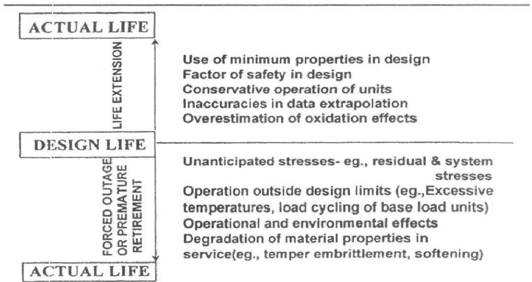
*Fig 6 : Factors that determine the "Actual Life" of Engineering Component*
