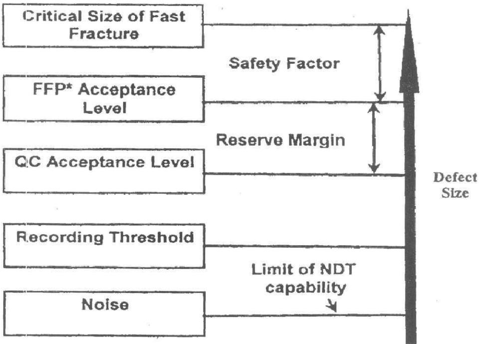
Fig. 1 : Defect size ranges covering quality (QC), FFP and NDT capability
