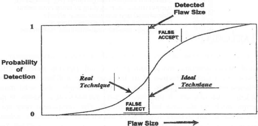
Fig 5: Probability of detection (POD) curve as a function of flow size for both ideal and real technique
