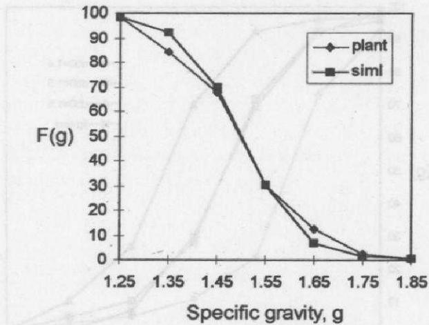
Fig. 3 : Comparison of partition behavior of a jig : plant vs. simulated data.
