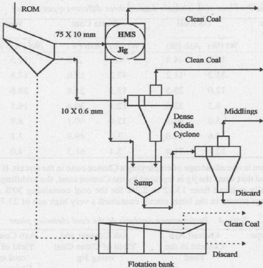
Fig. 5 : A typical coal washing flow sheet with two stage dense medium cyclones.
