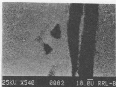
Photo 5 : SEM view of calcite in graphite flake.
