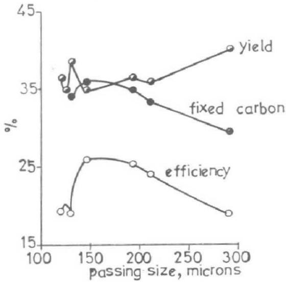
Fig. 3 : Effect of grinding time on flotation.
