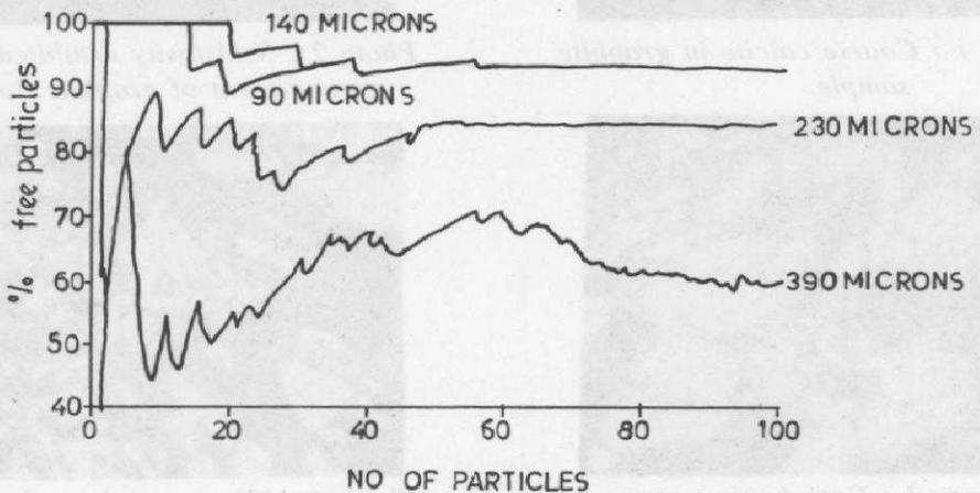
Fig. 2 : Liberation of graphite by grain counting using Faltsu method.
