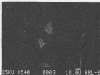
Photo 6 : SEM view of quartz in graphite flake.
