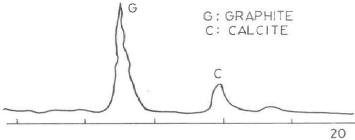
Fig. 1 : XRD pattern of graphite sample.
