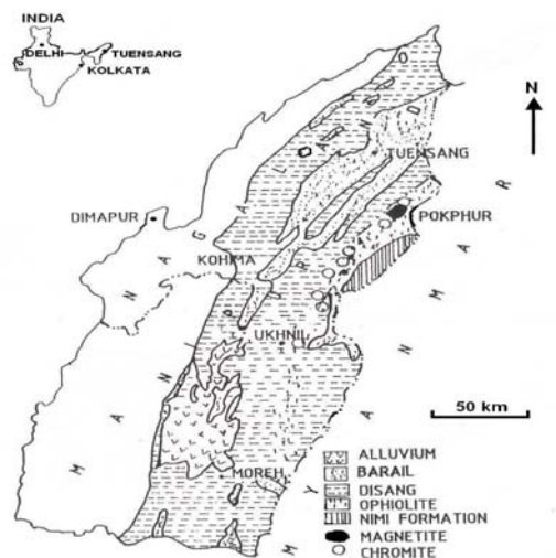
Fig. 1: Location of Pokphur magnetite body and regional geological map showing the disposition of ophiolite complex in northeast India.
