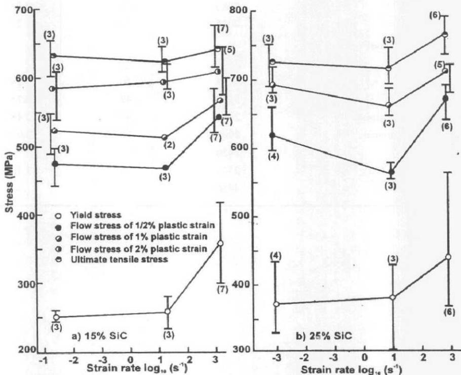
Fig. 2 - Effect of strain rate and volume fraction of reinforcement on the tensile yield stress, flow stress and ultimate stress of MMCs
