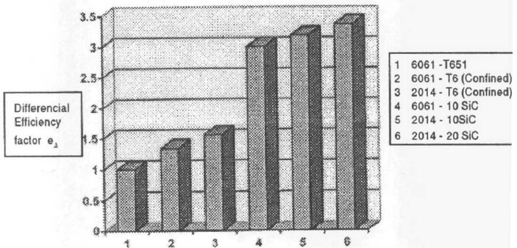
Fig. 6 - The differential ballistic efficiency factor for MMCs and unreinforced matrix materials [4]
