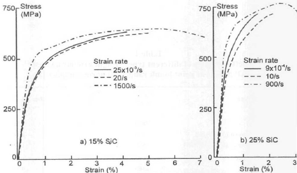
Fig. 1 - Effect of strain rate and volume fraction of reinforcement on the stress-strain curves of MMCs
