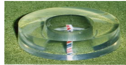
DT Cone for Hydro Turbine Diameter & Height ~0.5 mb
