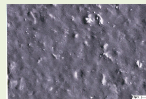
SEM photograph of a carbon-ceramic composite showing a protective layer at the surface
