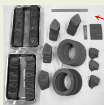
Different parts of clutch plate assembly fabricated at NOCCD, CGCRI, Kolkata
