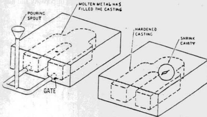
Fig. 2 : Shrinkage cavities
