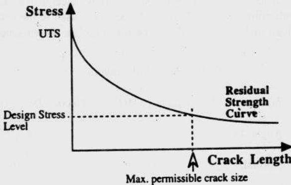
Fig. 6 : Decrease in residual strength of components on increase of crack length
