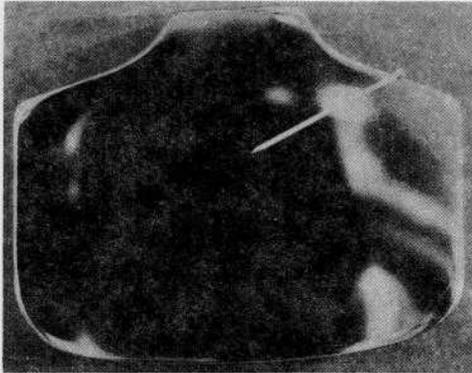
*Fig. 8 : Macrograph of polished rail head showing a vertical crack*
