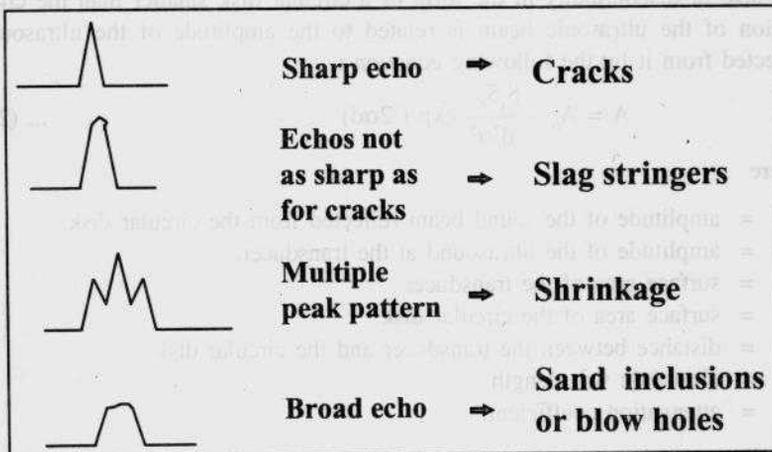
Fig. 5: Typical ultrasonic indications from four types of flaws found in castings
