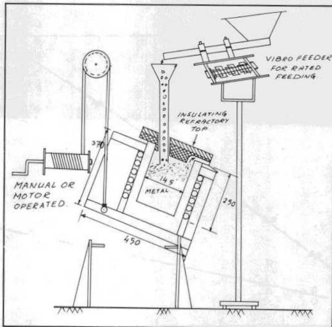
Fig.10 : Arrangements for continuous melting of sponge iron in induction furnace at NML
