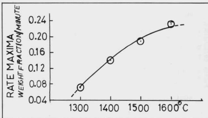
Fig.7 : Variation of the rate maxima with increasing temperature of molten pool in induction furnace
