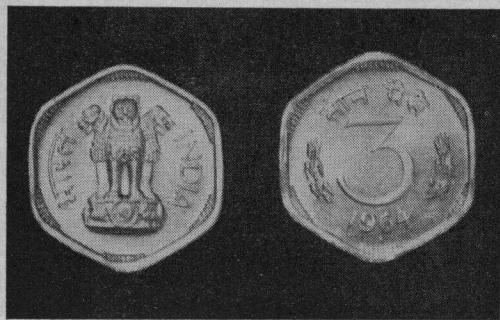
FIG. 33 — NEW 3 PAISA COIN MADE OF ALUMINIUM-MAGNESIUM ALLOY DEVELOPED AT NATIONAL METALLURGICAL LABORATORY AND GOVERNMENT OF INDIA MINT, BOMBAY
